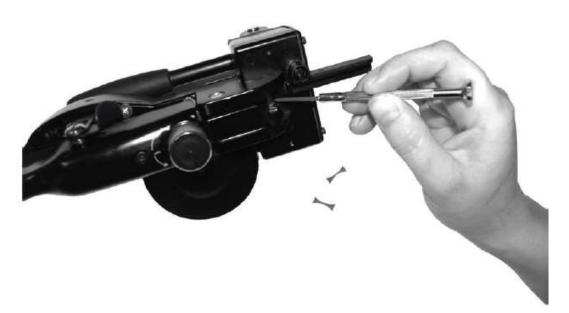
**CAREFUL!!!** Do not twist the wheel with pads (the one containing the characters) at the same time as tightening the actuation lever - the letters can be distorted, the tape can get stuck in the device, the pads can be damaged!
